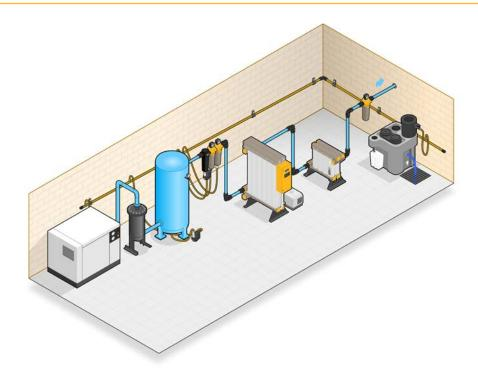
Heatless adsorption dryers (also known as PSA dryers) are the simplest type of adsorption dryer available and have long been the dryer of choice for many industries and applications. They are simple, reliable and cost effective and for small to medium flow systems, often
